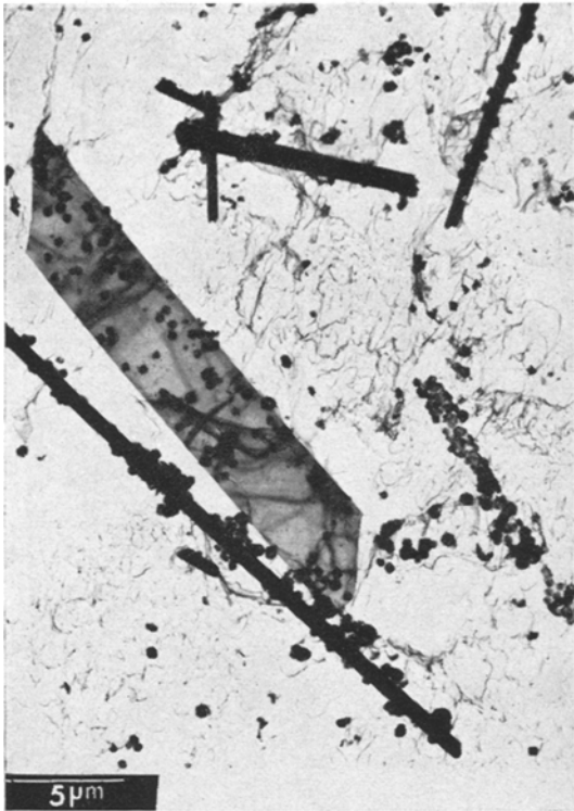
Figure 2 CTH whiskers after 120 h in Solution A.
