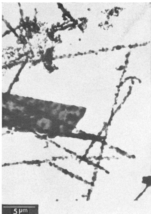
Figure 5 "Solution A treated" CTH whiskers after an anneal at 1100°C for 17 h.
