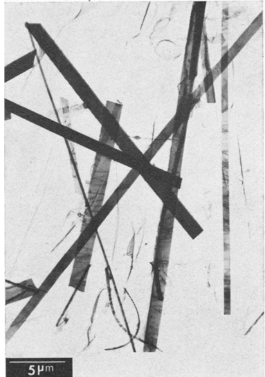
Figure 17 TFI whiskers after treatment in Solution A, water washing, and an anneal at 1100°C for 17 h.
